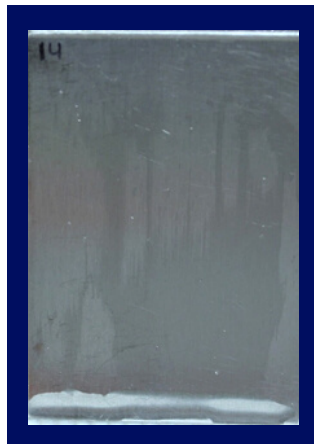
Common Failure - Water Break
