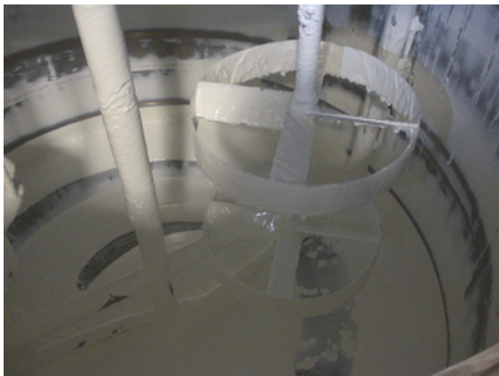
EQUIPMENT WITH RESIDUE CONTAINING HIGH AMOUNT OF TITANIUM DIOXIDE
