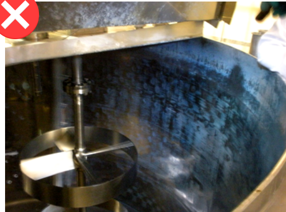
CLEANED WITH REGULAR ALKALINE DETERGENT. MANUAL SCRUBBING NEEDED TO CLEAN HAZE
