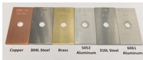
Coupons After 2 Week Test
